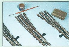
Above 1. The tiny screws can then easily be screwed into the baseplate through the switch housing using a jeweler's screwdriver.
