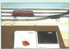
Test rolling stock in the hidden storage yard. The center studs and the rails have current connected to them to check that all the connections are working.
