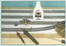
You can also test the current with a voltage meter. If everything appears to be working, the track is pinned down. White glue is dribbled between the ties, creating a durable adhesion without the need to screw down the track. The turnout motors are screwed down.
