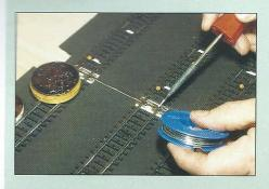
The joint between the front and rear segments is also achieved using Pertinax strips soldered onto the rails.
