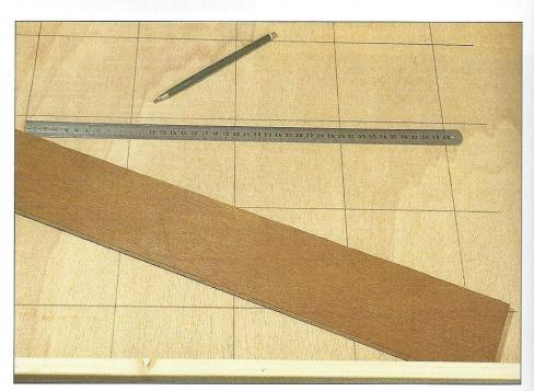
Before we start laying track, mark the layout segments from below with pencil lines some 10 cm (3-7/8") apart parallel to the outer edges. These lines will be a great help later on in laying the wires.
