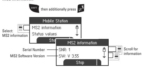
Here, you can get information about the serial number, software version, hardware version, locomotive data status, and Can Bus status.
