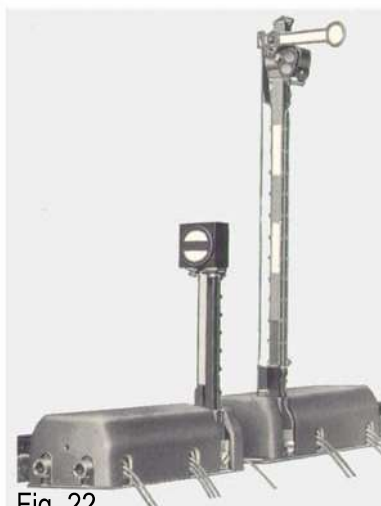
Fig. 22 Track blocking signal in front of a home signal at the exit from a station or yard
