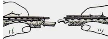
Fig. 10 Fitting the center conductor insulator 5022
