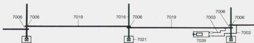
Fig. 13 Overhead conductor current interruption by two adjacent conductor wire insulators 7006
