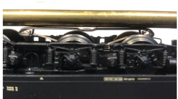
Fig. 8 – Noisy concave slider
