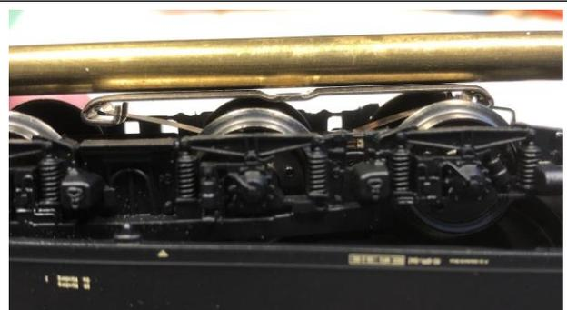
Fig. 9 - Quiet adjusted slider
