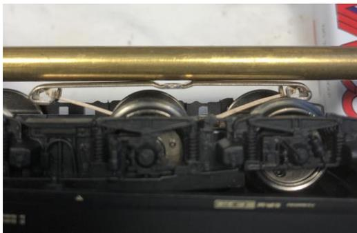
Fig. 7 - Noisy rounded slider
