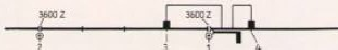
Fig. 7 Stretch of track with insulations at points 1 and 2 and installed contacts at points 3 and 4
