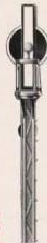
Fig. 15e "Push Off at Moderate Speed" obtained through blue cable with green plug
