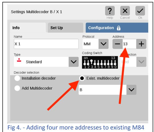
Fig 4. - Adding four more addresses to existing M84
