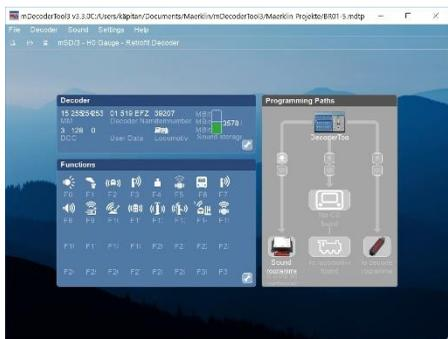
On the displayed dashboard you will find: Decoder, motor functions and programming paths. There are pre-set basic settings displayed. Click on the tool icon to change decoder settings. The other two windows allow you direct access when editing an existing project.
