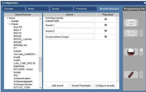
In the "Sound without Output" need a sound from the categories Anfahrt (arrival), Bremsen (brakes) (eg "Bachen / V200") or Schalten (switching). It is possible with more than one field "Sound without Output" to create and fill with sounds from the above categories. Sound without output is not among the maximum of 16 functions.
