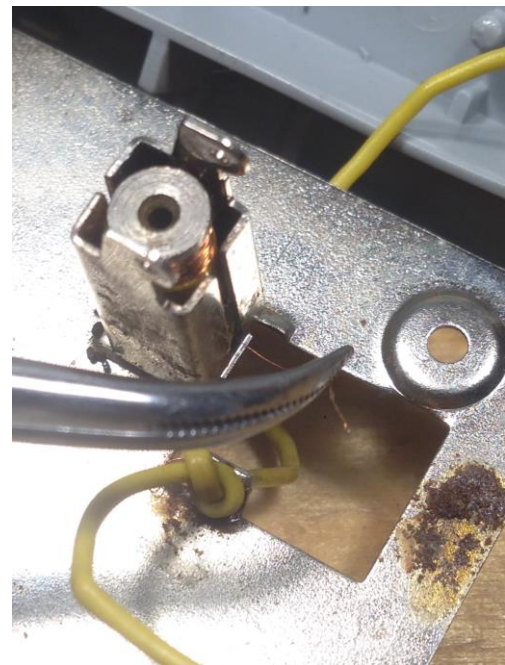
Fig. 5 - Varnished electro magnet coil wire
