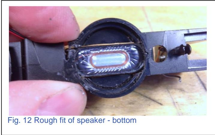
Fig. 12 Rough fit of speaker - bottom
