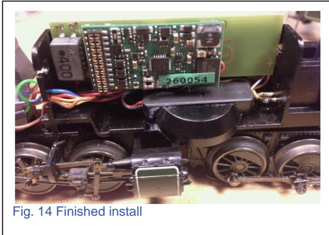
Fig. 14 Finished install
