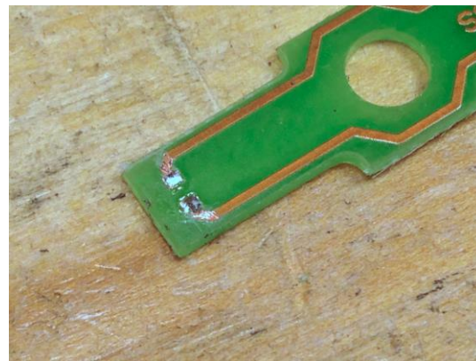
Fig. 17 LED removed and copper leads are scraped of varnish
