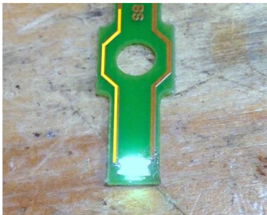
Fig. 18 New LED soldered in place and tested
