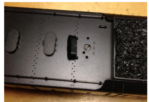
Fig. 1 Tender screw under hatch
