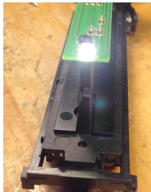
Fig. 22 New LED in place and tested
