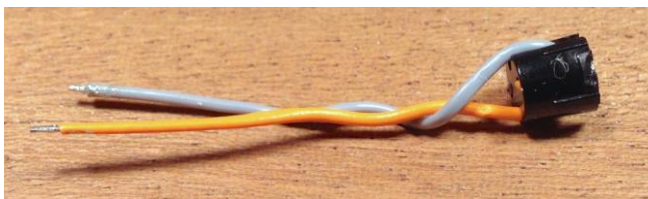
Fig. 7 Socket with wires, part #E276770
