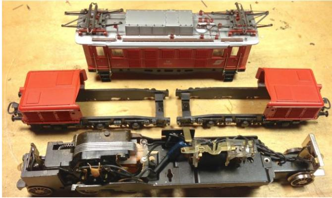
Fig. 2 - Locomotive body is removed
