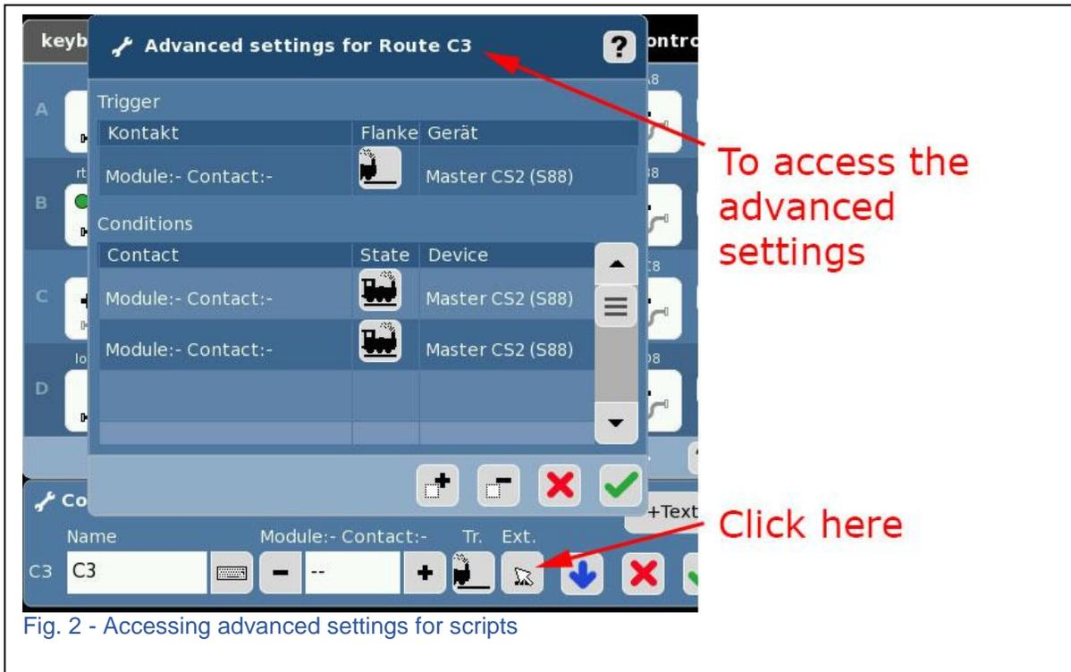
You can see the window is subdivided in two sections, the Trigger section (top) and the Conditions section (bottom). The trigger settings are identical to that of the settings next to the 'Ext' button (see very bottom of Fig. 2). It is now recommended that you always set the trigger settings in this window instead of the Configuration window, because the 'Gerat' or Device settings have changed when using newer L88/S88 with the CS2.
