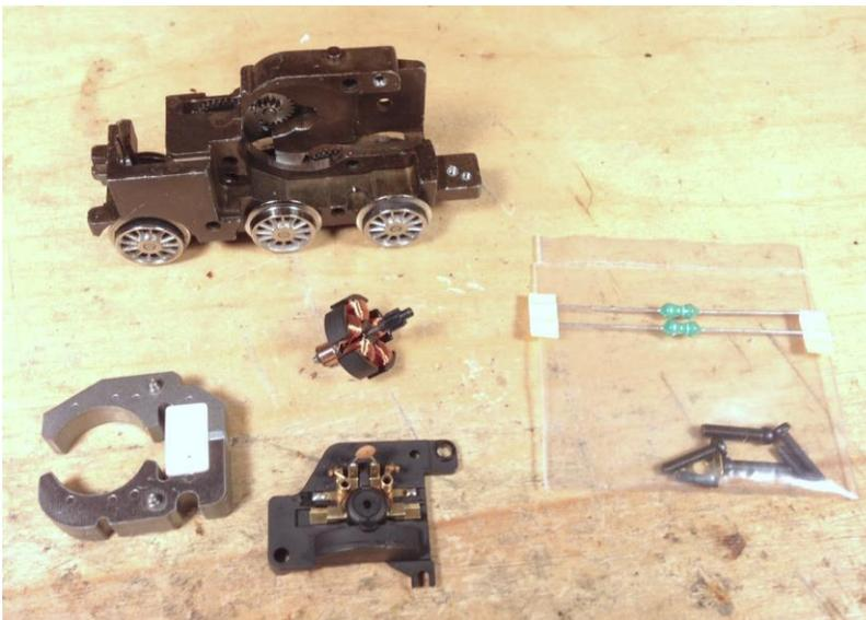
Fig. 4 - Motor components from 60944 set
