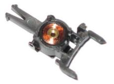
Telex coupling with coil removed (This is what you should see when the coil and PCB are very carefully removed together) - into the vacant cylinder, apply a thin strip of electrical tape (~2 mm x 14 mm)around its wall to provide a more firm seat for the coil.
