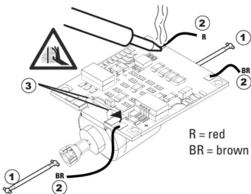
Loosen the motor from the circuit board.
