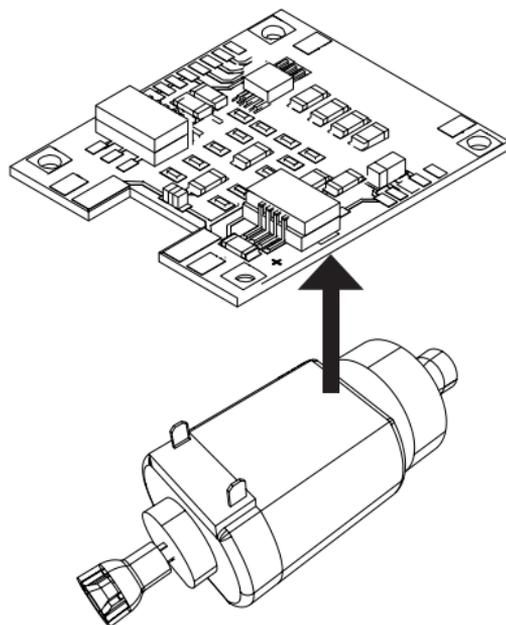
Lay the new circuit board on the motor, and carefully bend the solder tabs ① back into place. Solder the motor with both solder tabs to the new circuit board.
