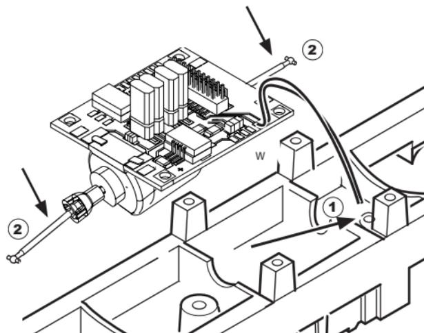
Screw the circuit board into place and solder the wires to it.
