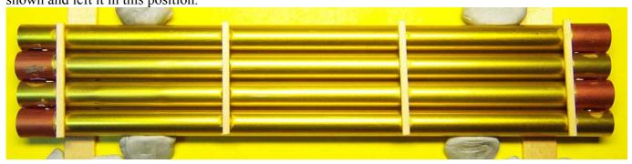
Taking one of the bottom layers orientate it until the collar positions are above the plain end of the pipes and glue it into place. Next glue the wooden planks at position above the existing planks, now orientate the last pipe layer until the collar positions are above the plain end of the pipes and glue it into place. Make sure the pipe stack is perpendicular and even in length.
