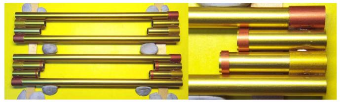
The two bottom pipe layers (left photo) were constructed on the work bench. The pipes rested on two (ice lolly sticks) and held in position with "Blu-Tack". The right photo shows a temporary spacer on the two
